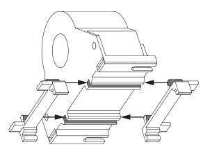
For horizontal DIN-rail mounting
