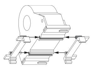
For horizontal DIN-rail mounting
